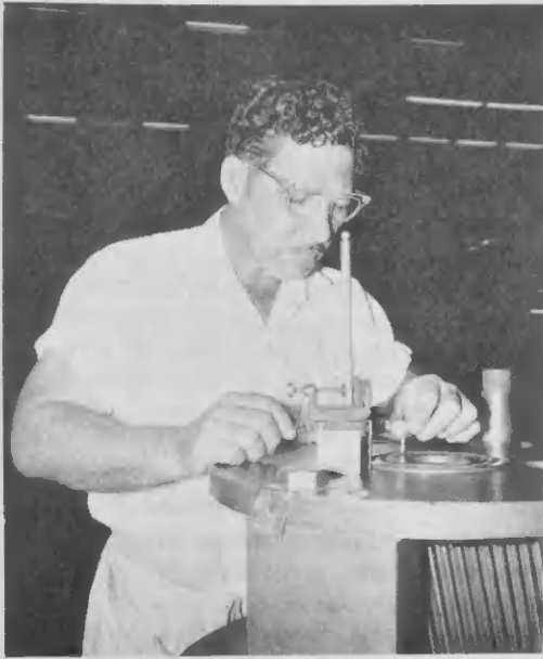
Francisco de Cuba uses protective glasses to check the end play of the gear of a mixer at the Machine Shop.
